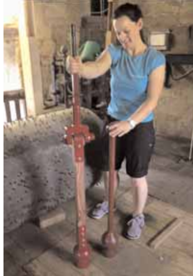
New wooden-shafted clapper and all steel one held by Leanne alongside the old tune barrel.
