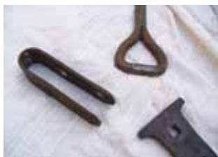
1. Main component parts forming the crown staple assembly.
