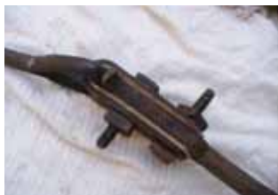
2. Completed crown staple assembly showing newly fitted baldric strap.
