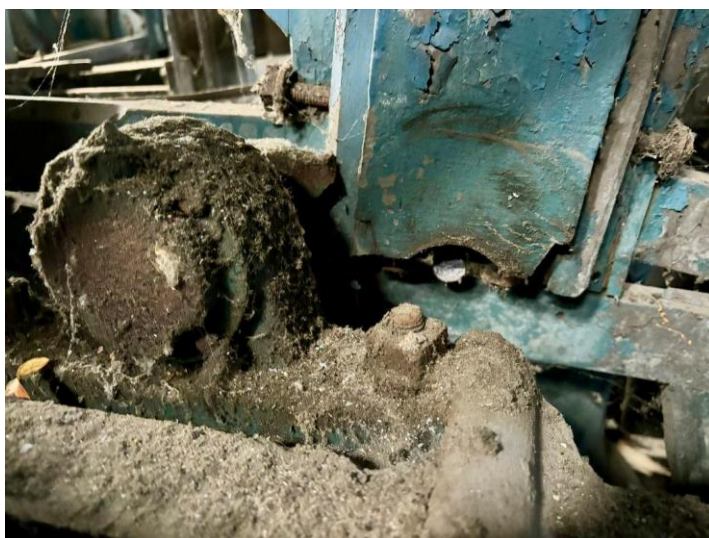
Broken gudgeon on the 5 th at Nuneaton
