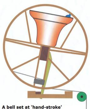
The stay holds the bell upright, with the slider blocked at the left. The rope goes over the pujlley and along the bottom of the wheel and is tied through the wheel at '8 o'clock'. The striped sally will be within the reach of the bell ringer below
